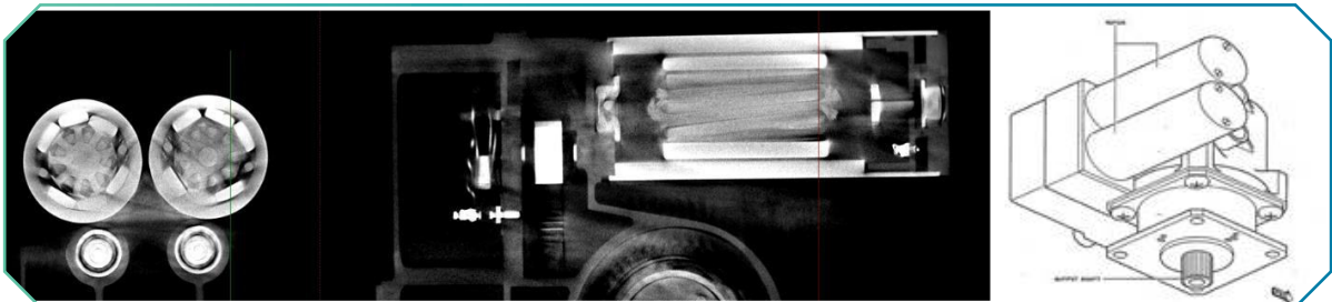
CT scan image showing motor A and B magnet disbonding
